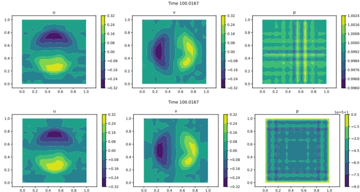
**Figure:** Simulation of vortex with source term at time  $T = 100$  with  $\mathbb{P}^3$  elements and  $6 \times 6$  cells. SUPG scheme (top) and SUPG-GF scheme (bottom)
